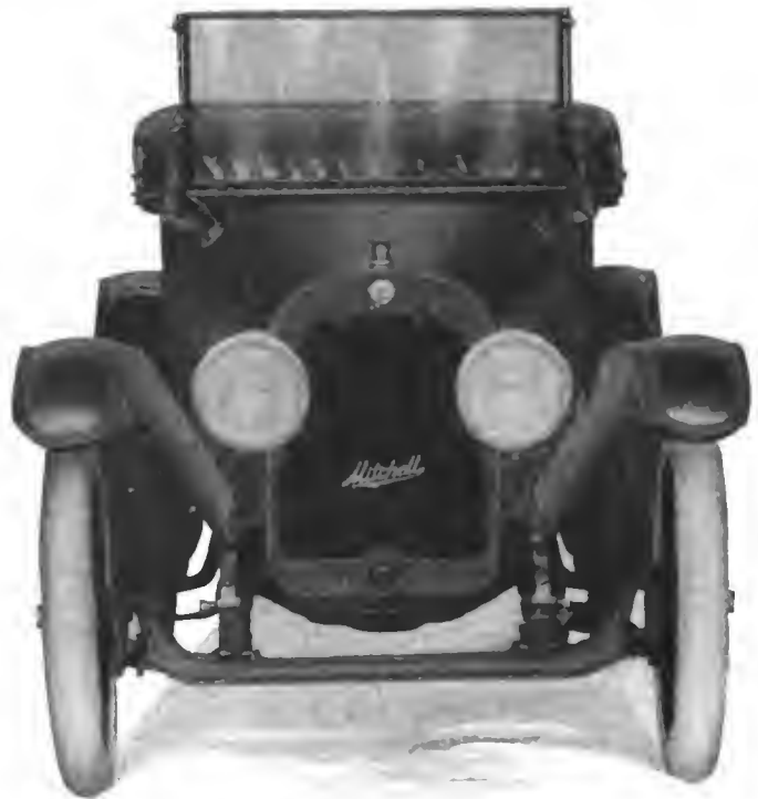
The front view of the new Mitchell six gives an excellent idea of the improved appearance in the body design. Note the high, narrow radiator and sloping lines of the hood
